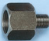
(1031 RF) inside thread G 3/8", outside thread M 10 x 1.0, fits between packer (1031), nipple (1120), stop cock (1170)
