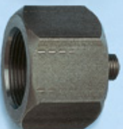
(1049 RF) inside thread G 1" to outside thread M 10 x 1.0 fits between packer (1049) and nipple (1120)
